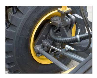
heel lean adjustment permits sound and safe work on embankments with no thrust loss from repeated steering adjustments, and guarantees precision tracking. On the all-wheel drive models, the front wheels are driven by a variable displacement pump and hub-mounted motors. The E.D.C.V. (Electronic Drive Control Volume) uses a hydraulic differential to match oil volume and, hence, the front wheel speed automatically to the speed of the rear wheels.
